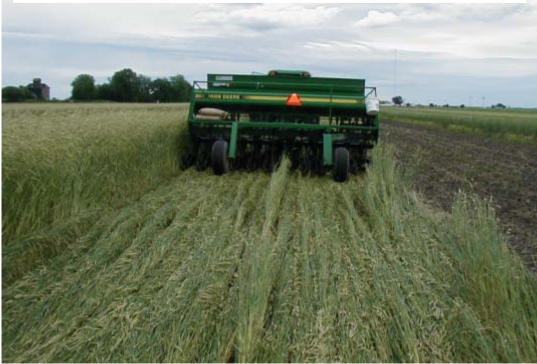
June 7, 2010 – planting soybeans into standing cereal rye with a JD 750 no-till drill
